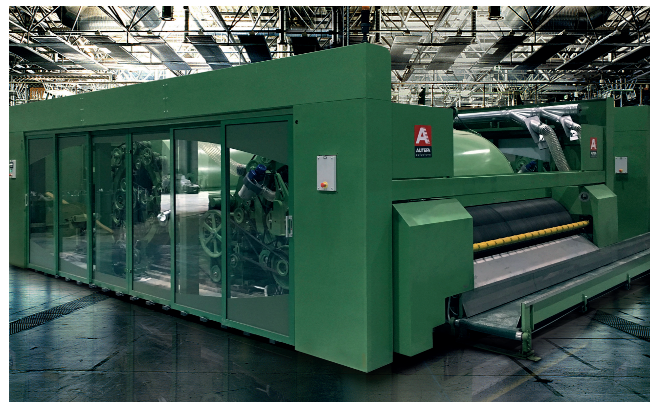
AUTEFA cards for processing wool and synthetic fibers for Woollen/Worsted-Semi Worsted technology
