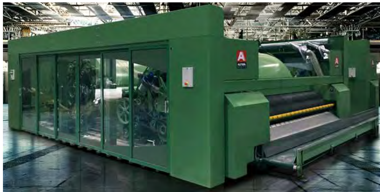
AUTEFA cards for processing wool and synthetic fibers for Woollen/Worsted-Semi Worsted technology
