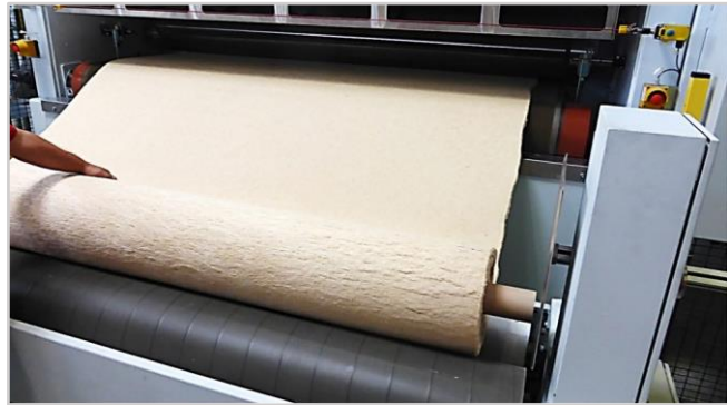
Winding station for the wood fiber nonwoven after a double belt heating system [6] (Bildquelle: TH Rosenheim)
