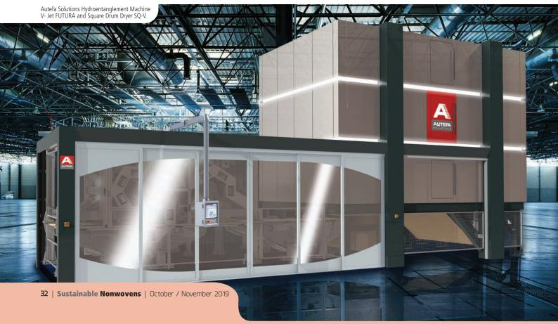
reduced to a minimum. Autefa Solutions Square Drum Dryer SQ-V combines the advantage of a horizontal belt dryer, and the better drying efficiency with the space advantage of a drum dryer resulting in increased drying length with small footprint.
