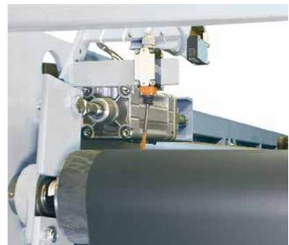
Belt 2 – tensioning and control system
