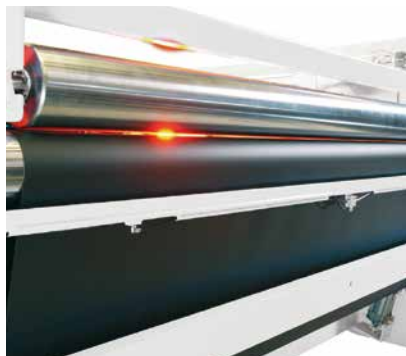
Belt 1 – 2nd web compressing roller
