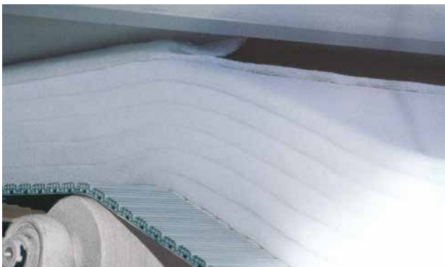
Crosslapper Topliner – controlled web laydown on edges
