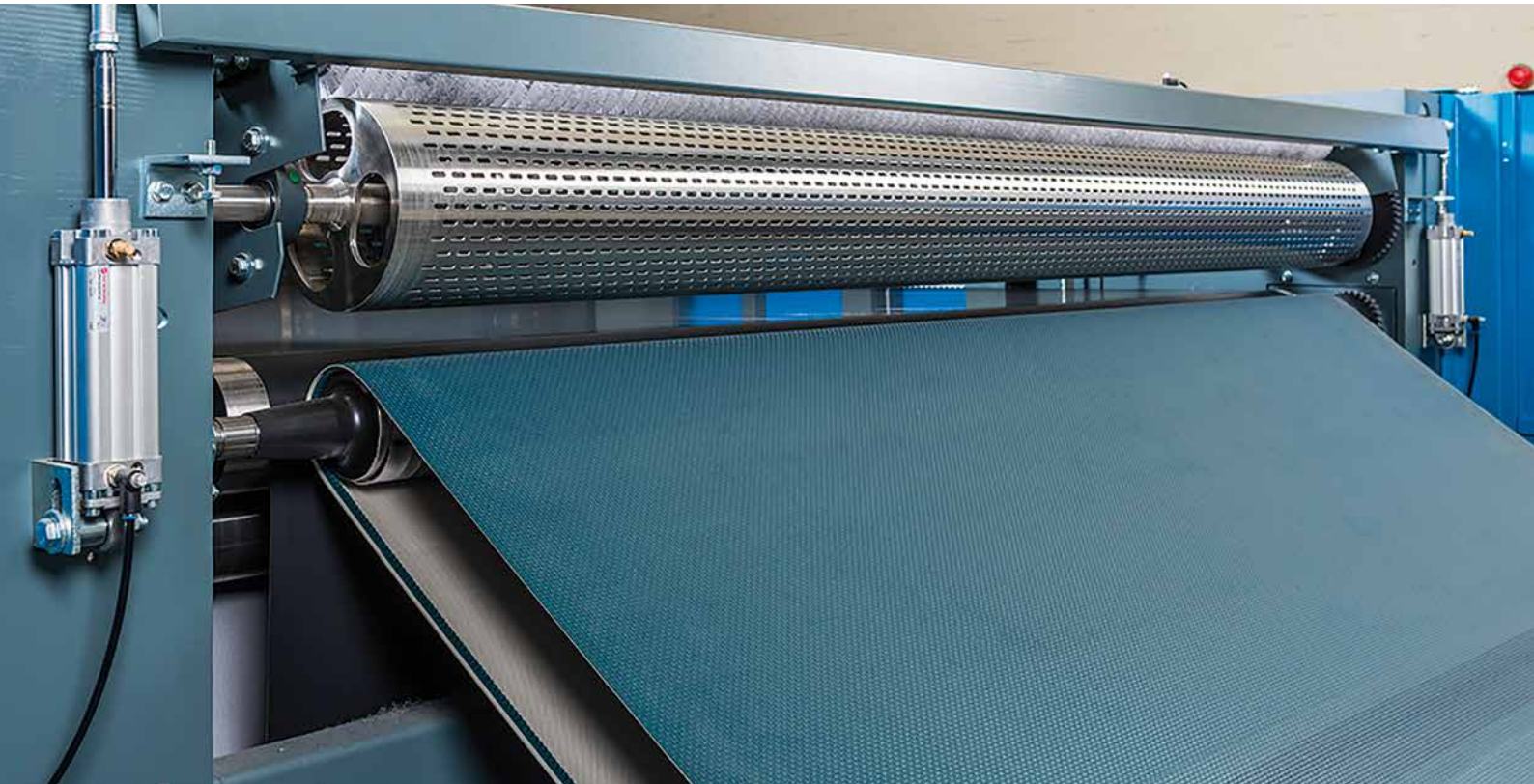
Crosslapper UnilinerONE – infeed belt
