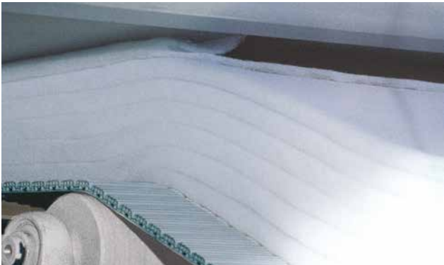
Crosslapper UnilinerONE – controlled web laydown on edges
