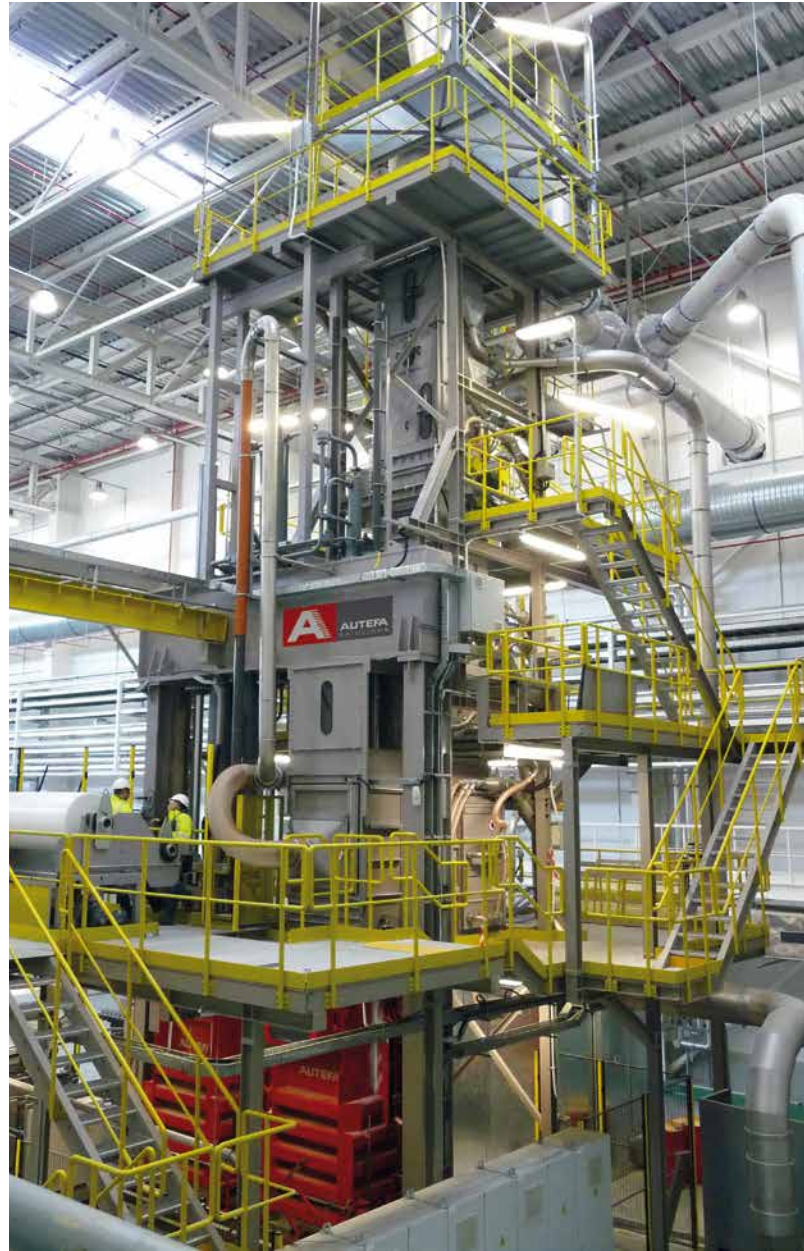
Short-cut baler with professional dust collection system
