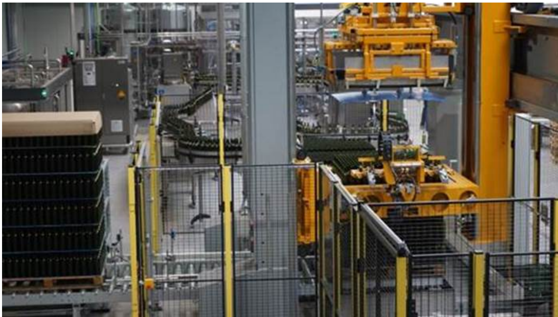
Sweep-off Depalletizer CERTANT R/"No-Broken Glass Device"
