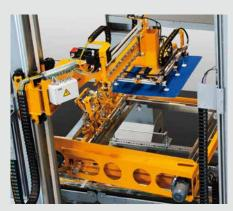
》竖瓶整层卸垛装置可整层卸垛各种圆形、 椭圆形、矩形的玻璃瓶、PET/HDPE塑料容器 或罐头容器至卸载传送平台上,然后传送至 灌装环节。 » The sweep-off depalletizer transfers layers of various configurations of round, oval, rectangular bottles, PET and HDPE plastic containers or cans onto a discharge table and leads them into the filling process.
